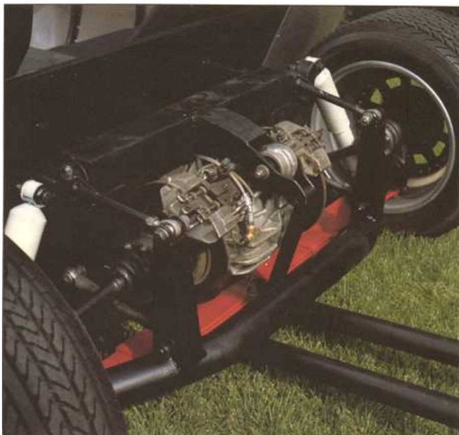
Rear end features: Alfa de Dion, brakes, 5 sp transmission-cum-clutch; note "Lawrence Spring" set off by "Tart's Bathroom" paint scheme.
