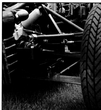
Dare we call it Lawrenceglide? From top: upper wishbones with inboard shock, brake driveshaft, "Lawrence Spring" with sway bar attachment and locating arm.
